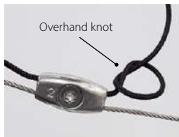
Restraint cable with overhand knots and end that is cut and melted after the cable clamp
