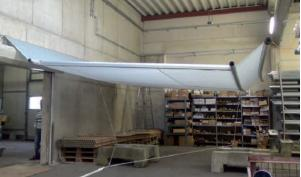
Photos: shadesign wind test – links: Strain relieved, right: Maximum load (shortly before end of test)
