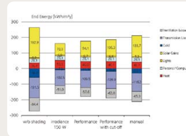
Fig. 11 Comparison of the specific annual end energy balance for different control strategies of the shading device. Here the results for the case with overhang for an requested illuminance level of 150 Lux are shown.
