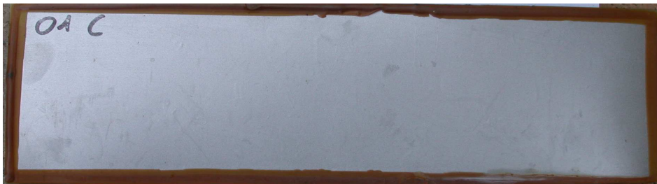
Fig. 2: 470LI at the end of the test (exposure period: 1000h); no pits observed.
